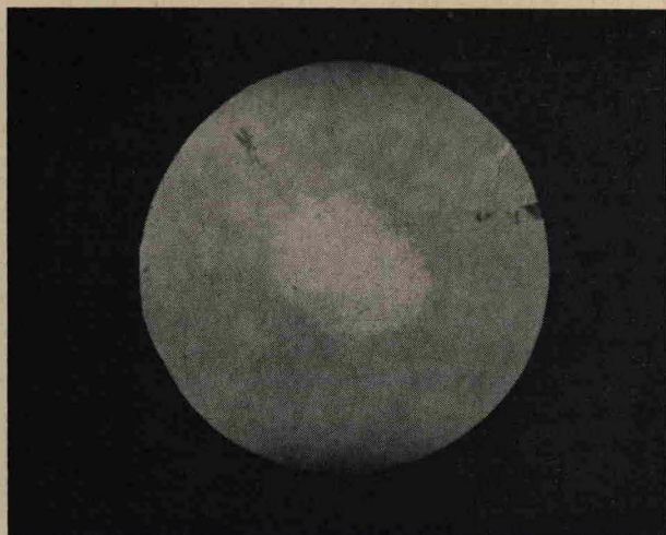
FIG. 6. Photomicrograph of iron under pressure in reflected light. The light area in the center is the high pressure phase.
